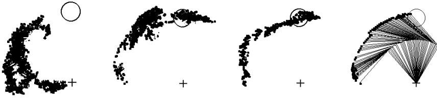
Fig. 4. The development of the reaching movement: from left to right, the arm first has an erratic movement; after a while, it occasionally comes through the reinforcement zone; the movement becomes smoother and smoother; finally, the arm has a direct and smooth movement. The cross indicates the shoulder of the arm. The circle is the reinforcement zone. In the 3 leftmost plots, the position of the hand is indicated. In the rightmost plot, the whole arm is sketched.
